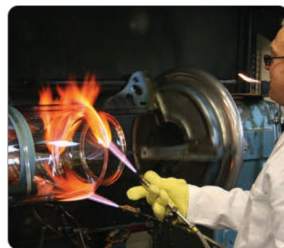
In-house design and manufacture of custom glass reaction vessels and frameworks
